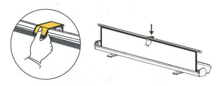
Close the casing and then rotate the left and right support plate to 90 degree.
