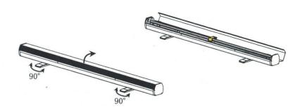
• Pull the handle indicated with the yellow label and pull the upward until the maximum height is reached
