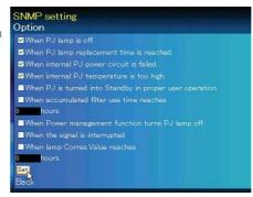
"When PJ lamp is off" signifies the lamp goes out without user operation. "When PJ is turned into Standby in proper user operation" signifies that the projector is turned on by using the web browser and then it is turned into standby with ON/STAND-BY button on the top control or the remote control.
