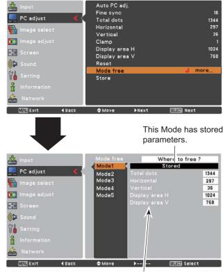
Values of Total dots, Horizontal, Vertical, Display area H, and Display area V.
