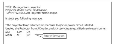
The projector lamp was turned off, because the projector power circuit failed. Unplug the AC power cord and plug it, and then turn on the projector once again to verify operation. If the problem still persists, unplug the AC power cord and ask servicing to a qualified service personnel with the error information.
